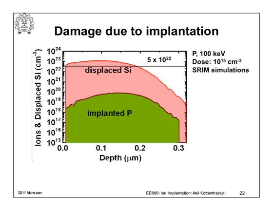
How much damage can be created by an ion? Typically an energy of 15 eV is required for creating a stable vacancy – interstitial pair. So we can assume that about 1000 such pairs are generated per ion implanted at 15 keV. The figure shows the density of displaced silicon by a phosphorous ion implant into silicon. The displaced or recoiled Si density is high near the surface and decreases as we go deeper into Si.
