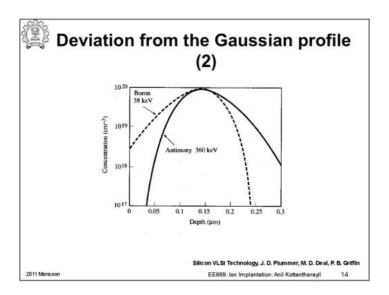
However the skew seems to depend on the ion. This slide compares the the profiles of B and Sb. The Sb implant is seen to be skewed more into the substrate.
