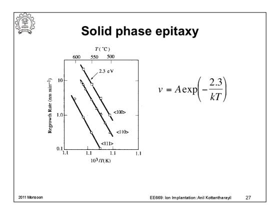
Solid phase epitaxial regrowth of the amorphous Si can be start from the amorphous-crystalline interface. This is a layer by layer regrowth of the crystalline structure from the undamaged template. The process can happen at temperature as low as 500C and has an activation energy of 2.3 eV. During the regrowth significant amount of dopant activation can also occur in the regrown region.
