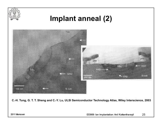
+1 defects when annealed may lead to clusters of interstitials in the {311} planes – experimentally observed. Three kinds of such defects are shown in these figures, namely End of Range (EOR) – at the edge of the amporphised region, Projected Range Defects (PRD) and Mask Edge Defects (MED).
