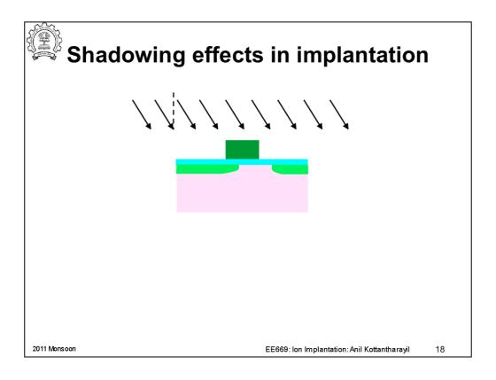
Tilt is represented in this image by showing the beam as being tilted. Typically the wafer is tilted with respect to the beam.
