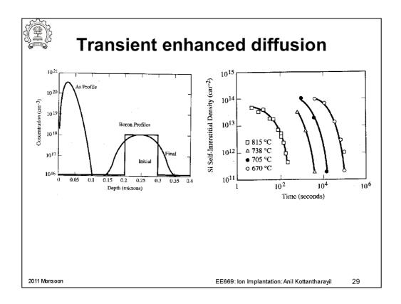
TED is a phenomenon in which during the implant activation a fast diffusion (~ 1000 X faster than normal) diffusion is seen during the initial phase of the anneal. The example on the left illustrate the point clearly. A boron retrograde profile is created in the Si by epitaxial processes. As is subsequently implanted into Si surface. The As implant creates significant concentration of defects in the surface layer.
