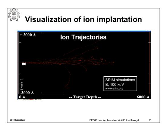
SRIM is a Monte Carlo simulation program for calculating the trajectory of accelerated ions in an amorphous material.
