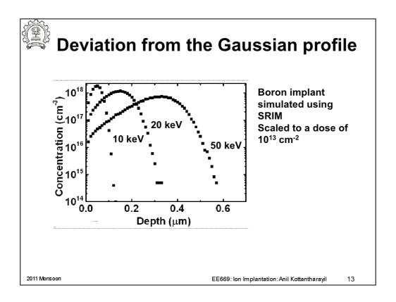
So far we had assumed that the implanted profile can be described using a Gaussian profile. This would allow us to make first order calculations of junction depth and peak concentration for a given energy. The same information can also be used for first order design of mask thickness for masked implants.
