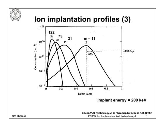
The figure shows the implant profiles for different common dopants. The implanted species in all the cases are the singly charged ions of the dopant atoms. The implant energy is 200keV. It is clear that the lighter the element, deeper it gets implanted.
