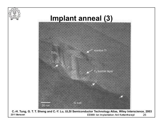
When  $\mathrm{BF}_2$  is used for ion implantation, fluorine bubbles may show up for high doses.
