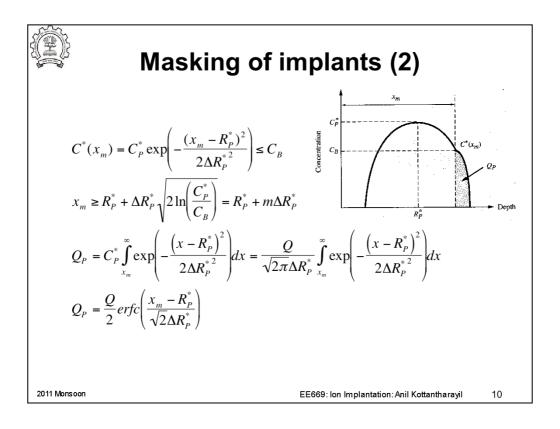
C\* is the concentration of the dopant in the masking material.
