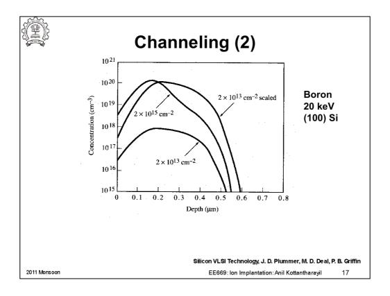
The slide shows the distribution of boron implants of different doses into (100) Si. If we consider either of the two doses, the resultant distributions can be thought of as composed of two distributions. In simulation software like Sentaurus, the distribution would be described using a dual Pearson distribution with 8 moments.
