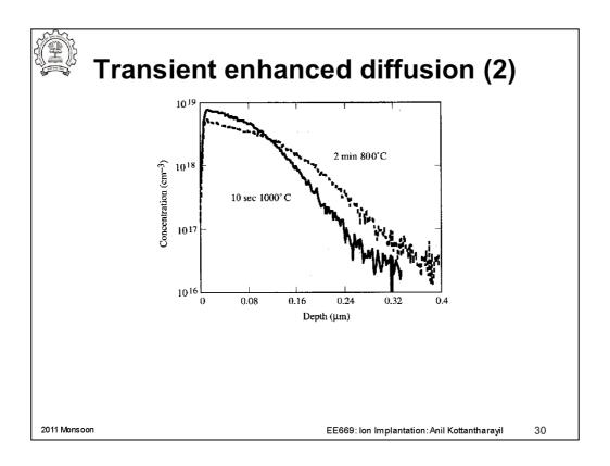
On reason to call this transient enhanced is that the defect annealing at high temperature can happen quite fast. So once all the defects are annealed, the diffusion would slow down.
