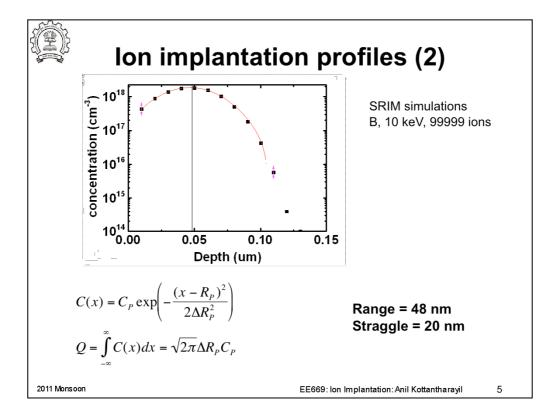
The figure shows the implanted profile perpendicular to the wafer surface along a line passing through the point of implant. The equations describe the Gaussian function which approximately represents the implant profile. The total dose implanted can be calculated by integrating the implant profile.
