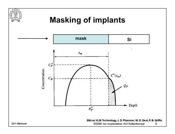
The idea of masking is to implant the dopant only in regions where we want to have them. However the ions would be also implanted in the masking material and a certain fraction of the dose can be expected to be implanted into the silicon as well. The mask thickness should be designed so that the tail of the distribution in silicon should not have a peak exceeding a specified value,  $C_{\rm B}$ .
