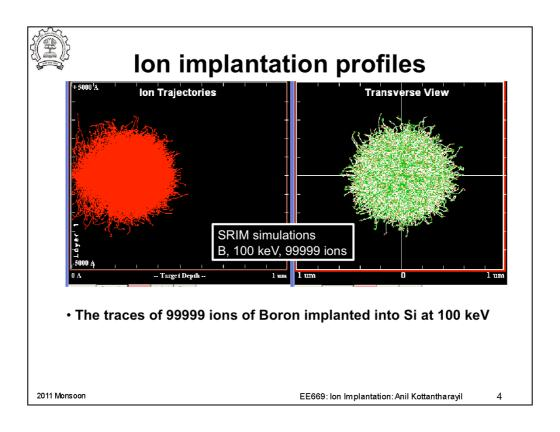
The ions are implanted at the centre of the vertical axis of the left figure. Even though the ion trajectory on the average has a preference in the direction of implant, the individual ions would be scattered in all 3 directions.
