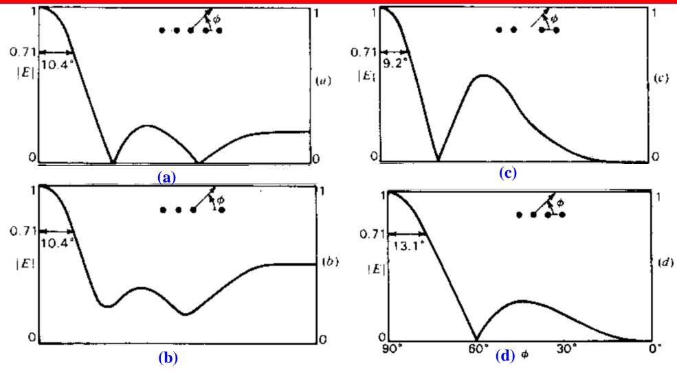
Radiation Pattern of linear array of 5 isotropic point sources of equal amplitude and  $\lambda/2$  spacing (a) all 5 sources ON (b) one source (next to the edge) OFF (c) one source (at the centre) OFF, and (d) one source (at the edge) OFF
