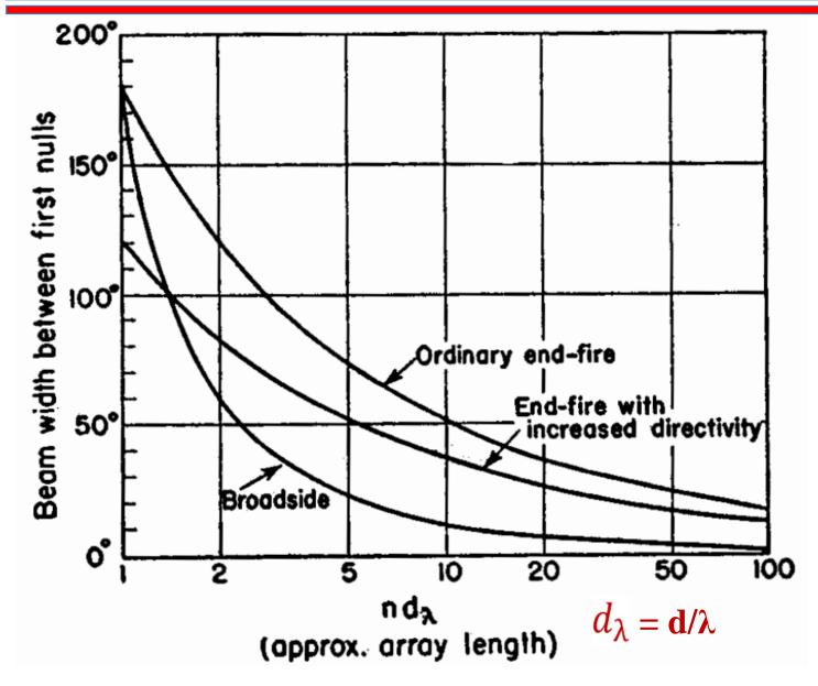
For long array, (n-1)d is equal to array length L
